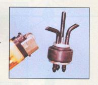
The three silicone fuel tubes must be fitted to the tank before it is installed on the fuselage. They need to be about six inches long and colour coded (the fuel feed needs to be easily identifiable) so that you
