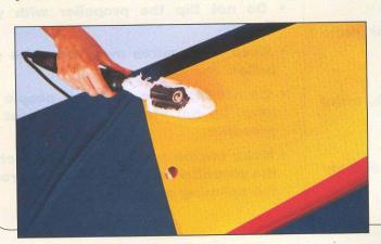
Use an iron covered with a cloth! Start at low setting. Increase the setting if necessary. if it is too high, you may damage the film.
