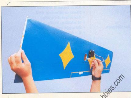
Separate servos are used for the left and right hand ailerons and you will need extension lead (approx 300mm long) and a short "Y" lead to connect the servos to the receiver. You could use one "Y" lead with long leads but this could make the routing of the leads much
