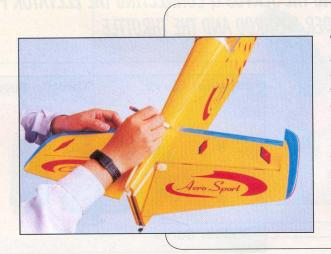
With the tail correctly aligned made the shape of the fuselage on the top and bottom of thr tailplane use the pen and draw lines onto the stablizer where it and fuselage sides meet do this on both the right and left sides and top and bottom of the stablizer
